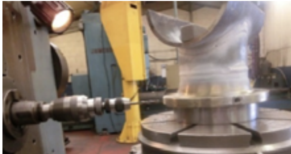
Bogie frame alignment machining
