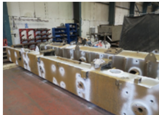
MPI on large components
