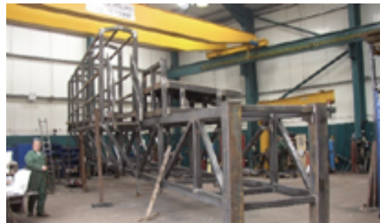
Fully manufactured Offshore Manipulator Arm assemble and factory acceptance tested.
