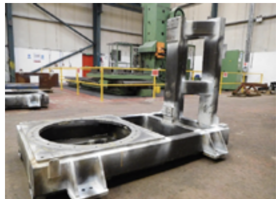
MPI on large components
