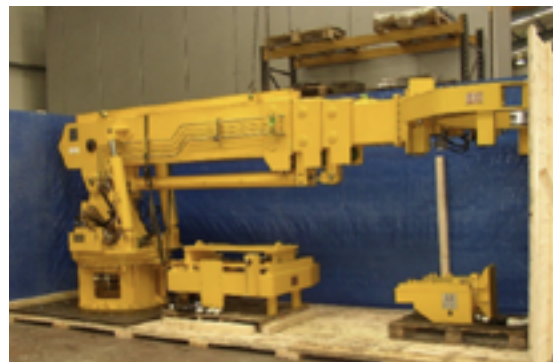
Fully manufactured Offshore Manipulator Arm assemble and factory acceptance tested.
